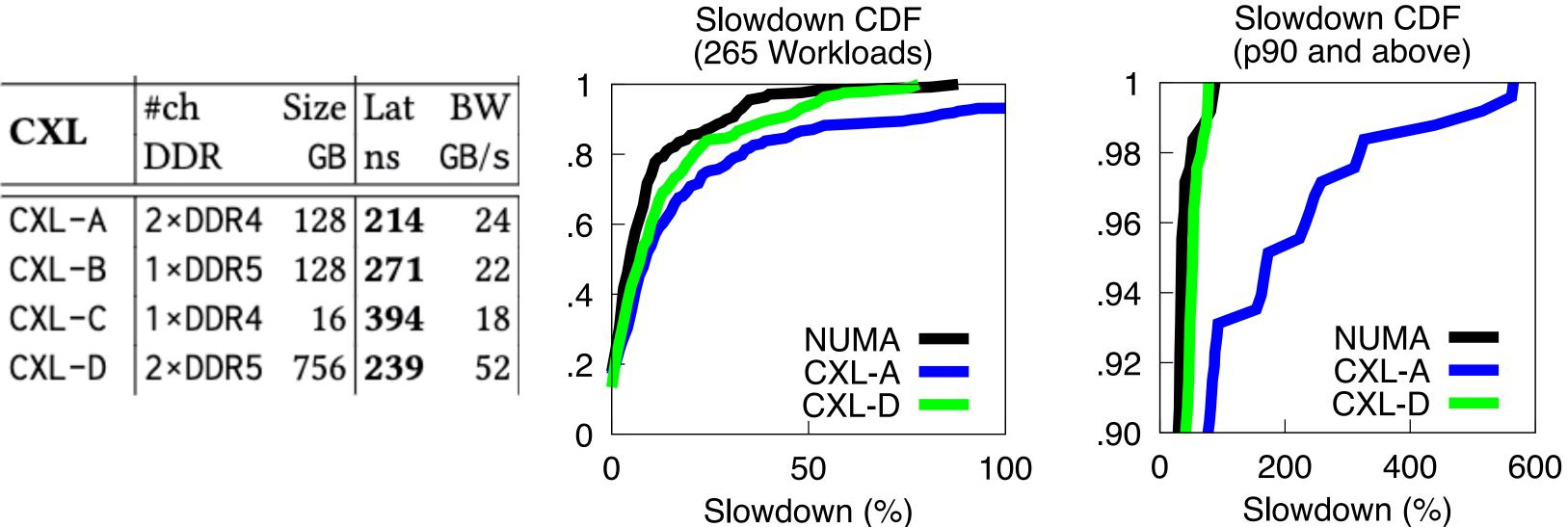
The bandwidth limitation on CXL causes some workloads with high slowdown. The performance gap between CXL(-D) and NUMA diminishes due to its higher bandwidth even though its latency is worse.
